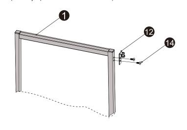
3. 2. 2 Installation for inner frame(Fixed by 2 pcs of allen screws)
