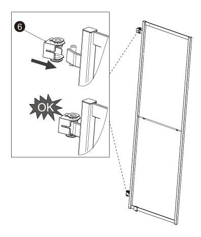
$3.2.2\,$  As illustrated below ,install the side frame step by step per installation below.
