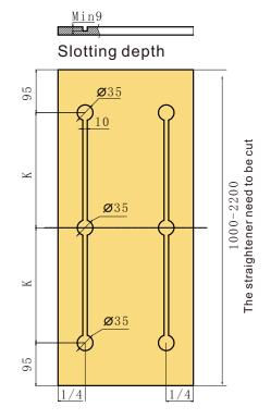
2. Straightener length cutting specification (When door height is 1000-2200mm)
